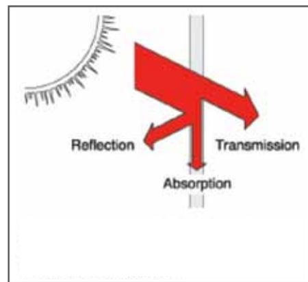
Figure 2.2: Solar radiation through a glazing material is either reflected, transmitted or absorbed
